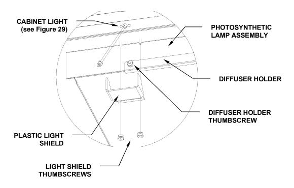
Figure 30: Replacing Photosynthetic Lamps
