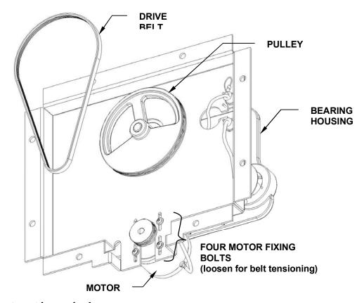
Figure 35: Belt Replacement & Adjustment
