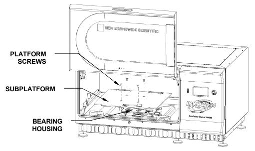
Figure 10a: Installing Subplatform
