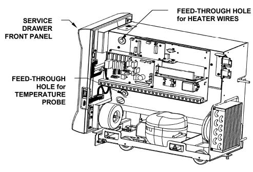
Figure 32: Service Drawer Feed-Through Holes (Germicidal Lamp Replacement)
