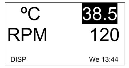
3. Turn or spin the Knob to reset the setpoint (in this example, turn the Knob left to decrease the setpoint to **37.0**).
