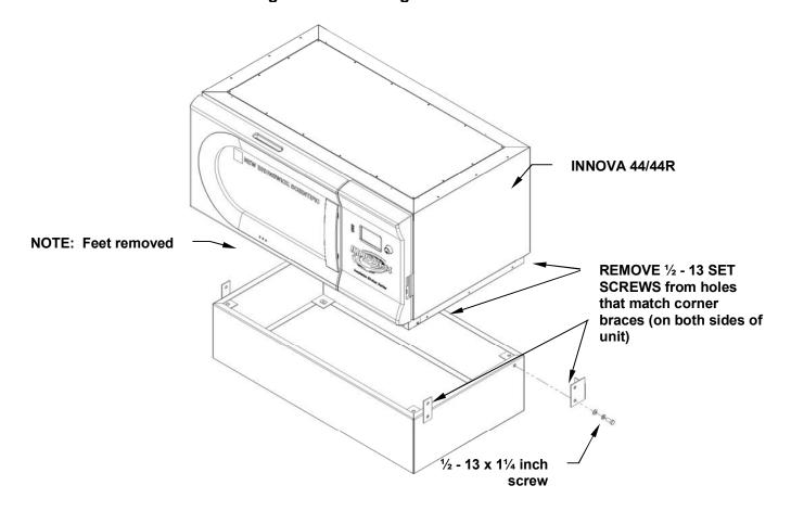
Figure 3: Mounting Shaker on Base
