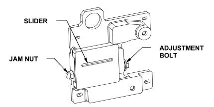
Figure 31: Righthand Counterbalance Bracket
