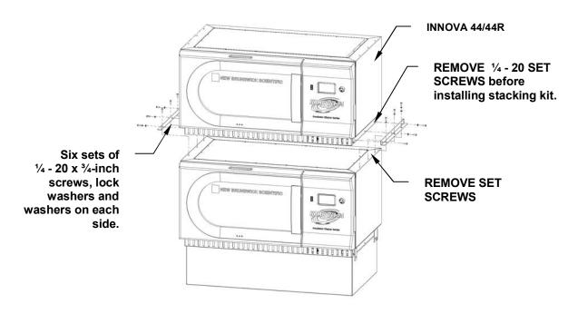
4. Using the screws and washers provided, attach the stacking kit mounting brackets to the top of the bottom unit. Secure the brackets in place as shown in Figure 5a above.
