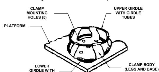
Figure 11a: Double Girdle Clamp Installation
