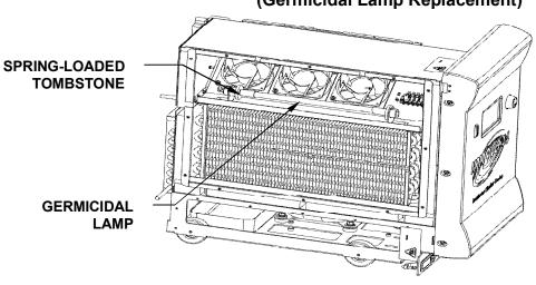
Figure 33: Service Drawer, Fan Cover Removed (Germicidal Lamp Replacement)
