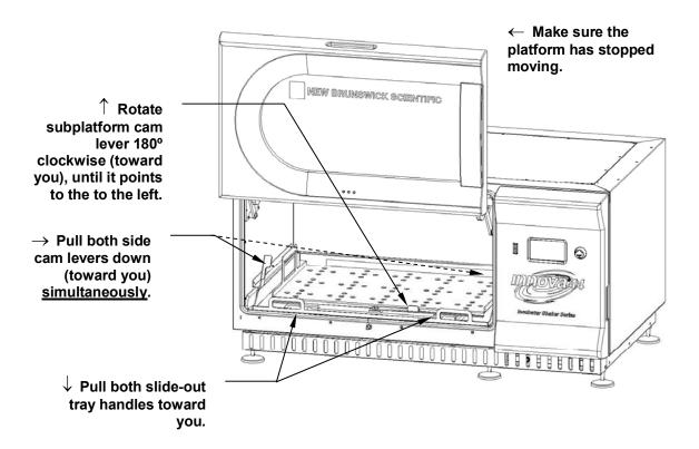
Figure 27: Disengaging Slide-Out Platform
